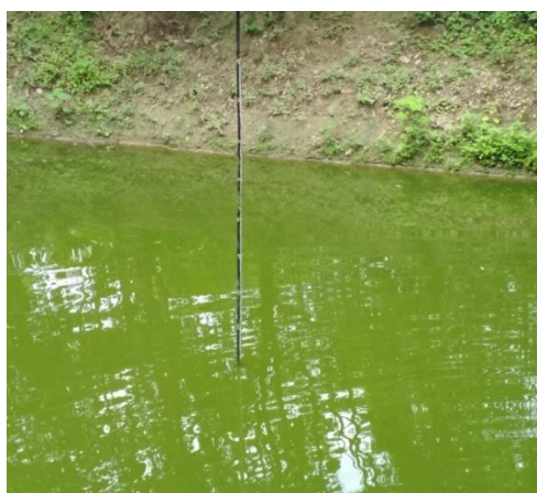
Figure 3.5: Water depth monitoring pipe
