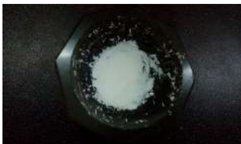
Figure 2.7: Sample preparation for FTIR
