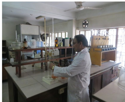
Photo 23: Titration for Crude protein determination of broiler meat
