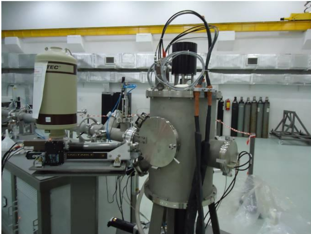
Plate : 2.3 Experimental Chamber of Tandem accelerator
