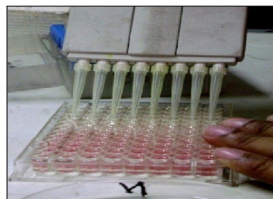
Figure 2.1.11 GOD-POD reagents being added to all the samples for determination of glucose.
