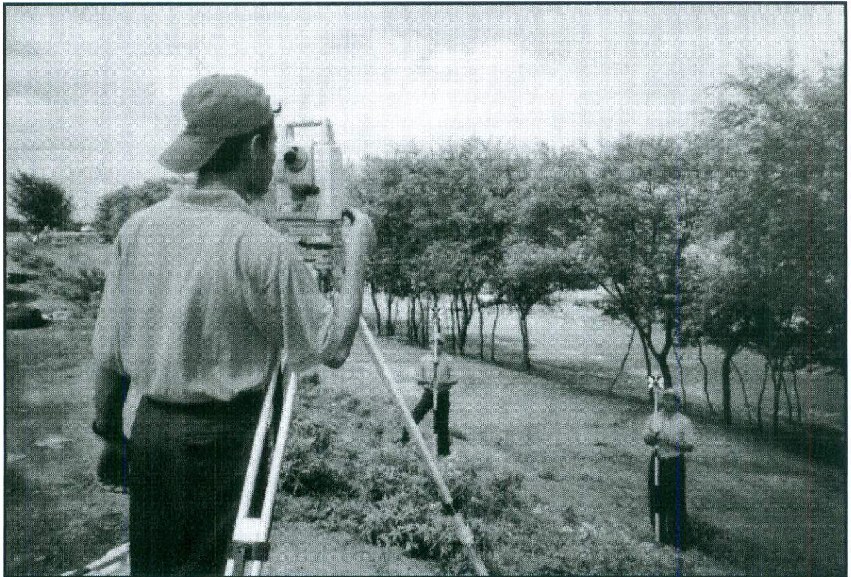
Figure 3: Typical Total Station Survey Set-up for Land Level Survey.
