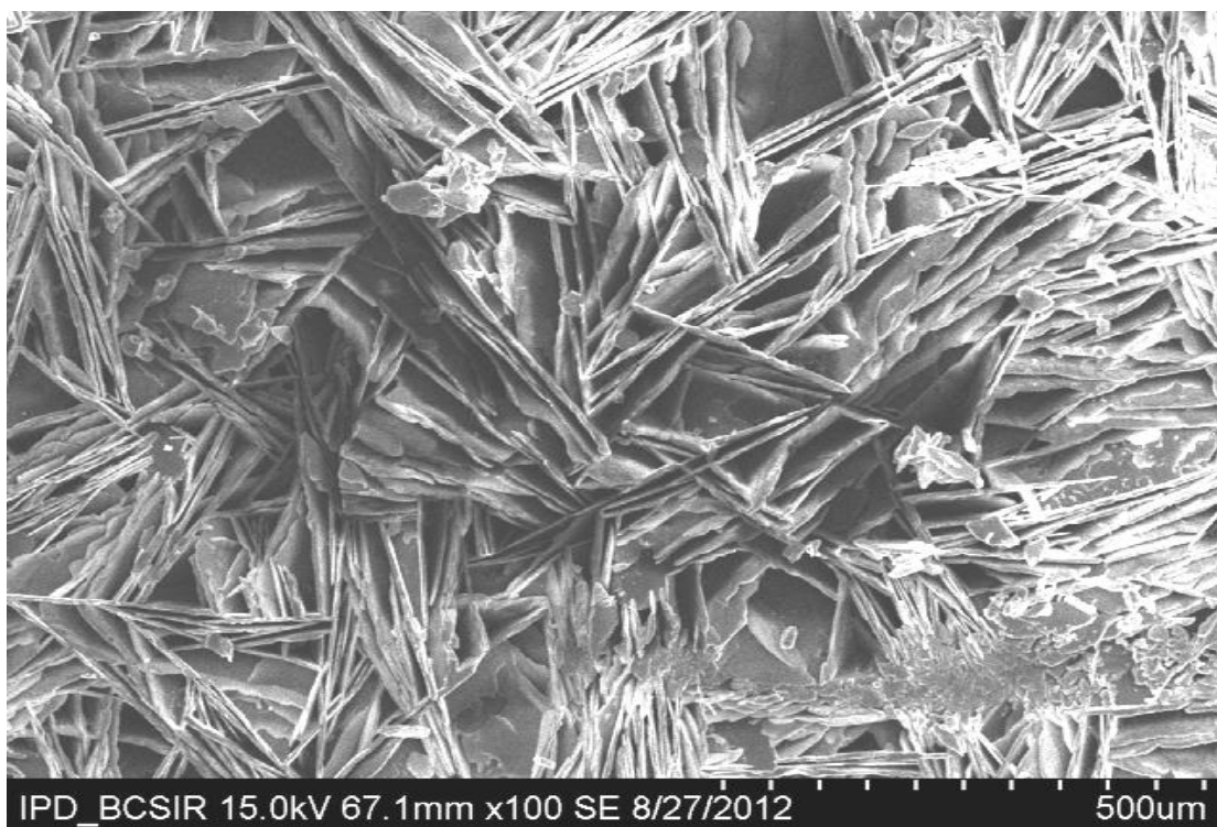
Fig. 10.5 Scanning electron micrograph of a 500 \mu\text{m} of sonicated dispersion of Starch-Ionic surfactant (SDS) complexes, SEM of magnification 100 times in Bar represent 500 \mu\text{m} .
