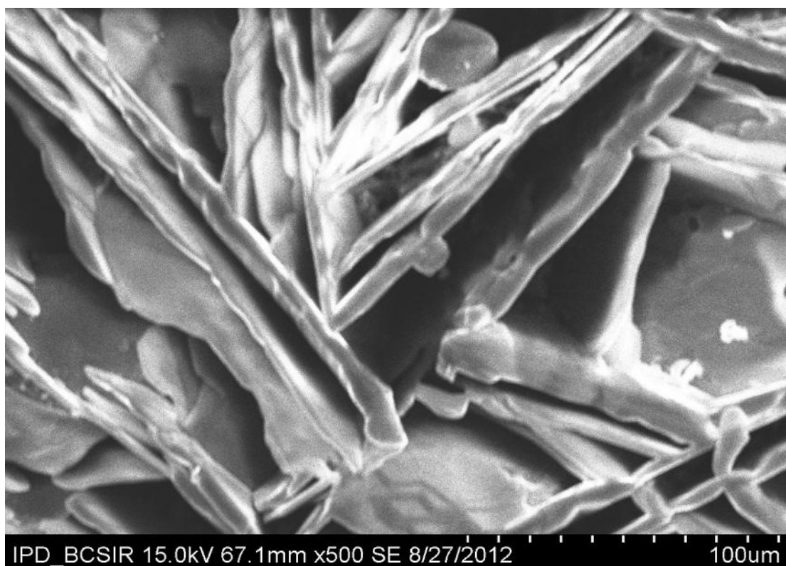
Fig. 10.7 Scanning electron micrograph of a 100 \mu\text{m} of sonicated dispersion of Starch (amylose) in presence of surfactant of CTAB SEM of magnification 500 times in Bar represent 100 \mu\text{m} .
