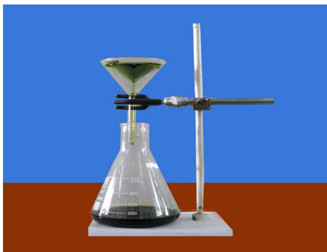
Plate10: Filtration of pet. Ether, acetone, chloroform and methanol extracts.
