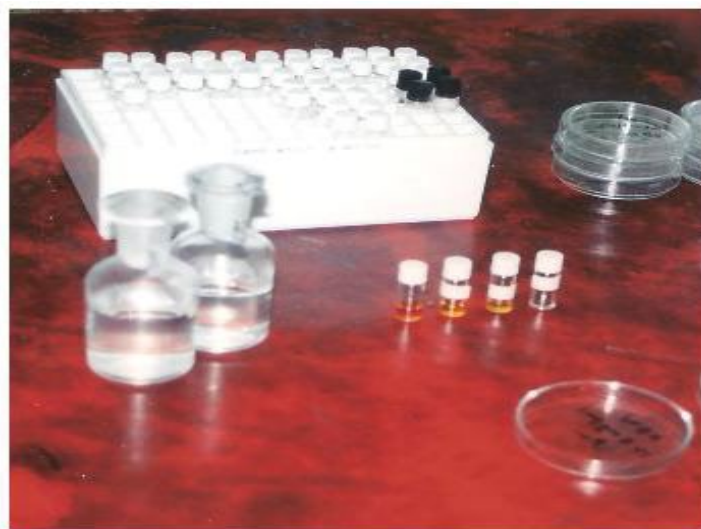
Plate 15: Preparation of doses for surface film test
