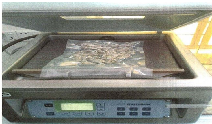
Plate 7.1 Vacuum and N 2 packaging by Multivac packaging machine
