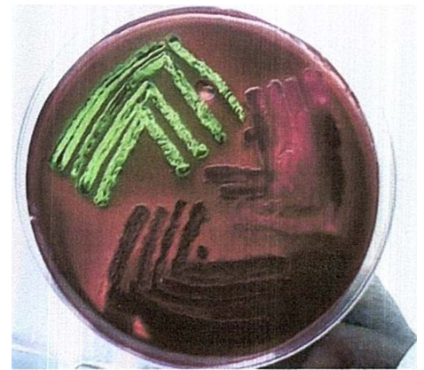
Plate 5.2 Colonies with green metallic sheen for fecal coliforms in W. attu of traditional sample
