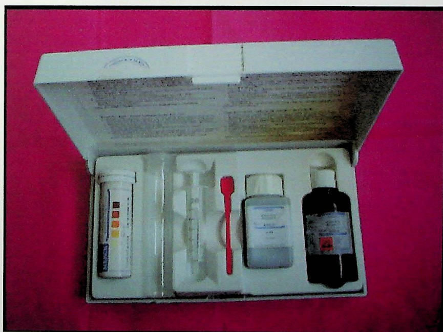
Figure 4.2: Inner view of Merck arsenic test kit
